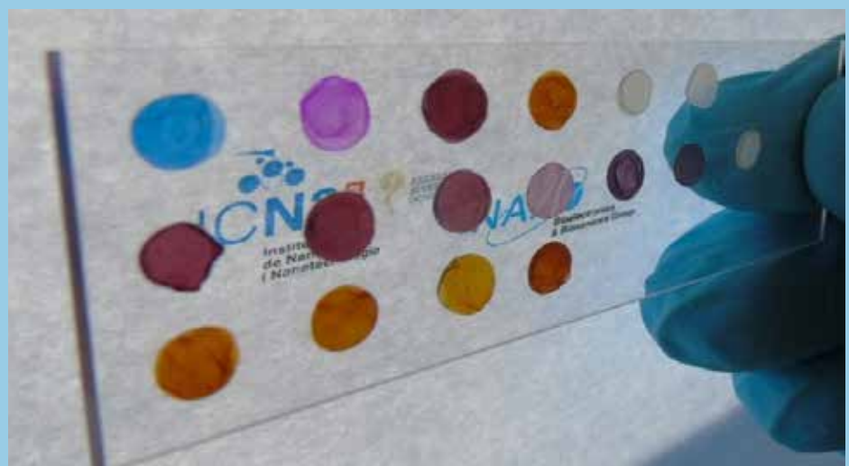
Printed bacterial cellulose nanopaper for biosensing applications, presented by Catalan Institute of Nanoscience and Nanotechnology at ESMA's AFIP conference in March 2016
